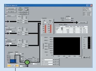
**HOVACAL** is available as a digital and an analog version. The digital HOVACAL is an autonomously running device and can be operated remote with the software viewCAL and an external PC. HOVACAL digital is able to mix up to three span gases with a vaporized liquid.
